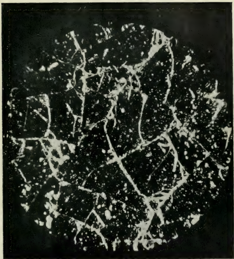
MICROPHOTO OF MASTIC VARNISH, SHOWING CRACKS.
